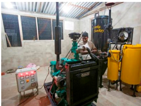
A 12 KW Biomass Gasifier Generator developed and manufactured in Sri Lanka
